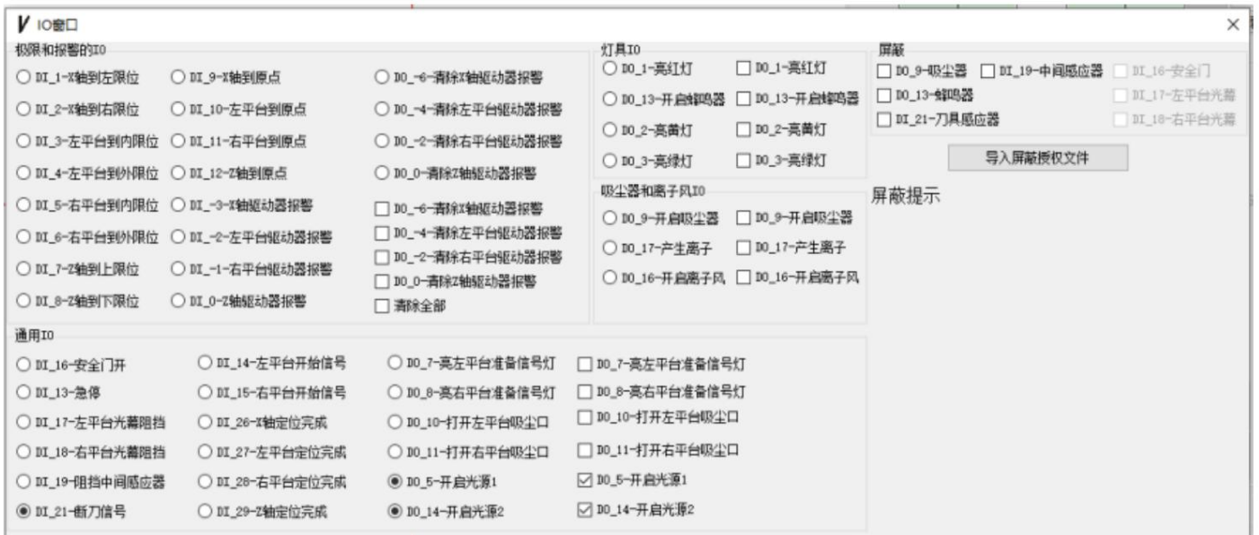
IO Window: This interface displays the status of each axis, the positive position of the limit switch, and the limit switch status.
